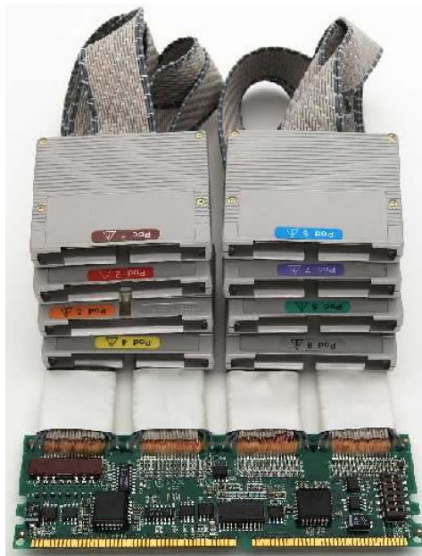
Figure 15. Custom Logic Analyzer Probe for DDR266 from FuturePlus Systems
