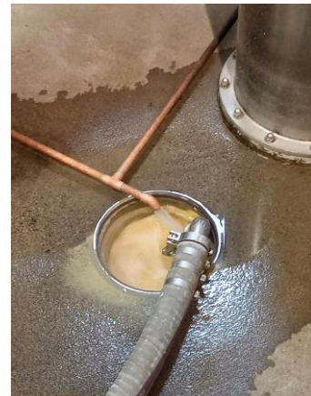
Spent Wash being discarded into the drain while being cooled
