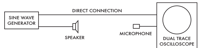
Figure 6.7 Apparatus setup for measurement of wavelength.
