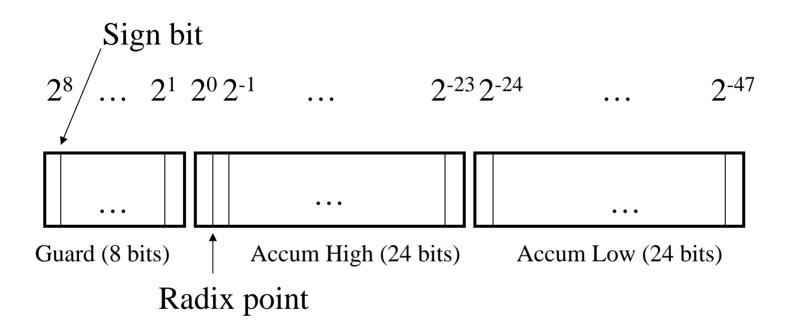
Motorola 56xxx has two 56-bit accumulators (48-bit result with 8 guard bits)
