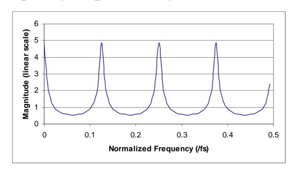
• A "comb" filter. Frequency at peaks depends on delay length.
