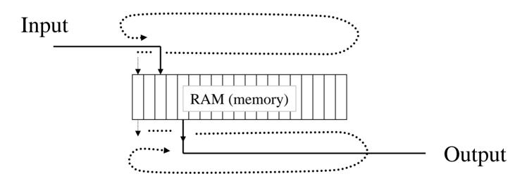
...and read out later. Delay is the number of samples between *write* pointer and *read* pointer.
