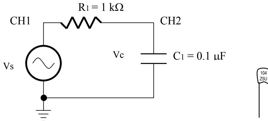
Using a sine wave from the function generator with peak-to-peak amplitude of 2 volts, fill out the following table.
