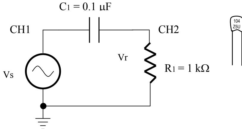
Again using a sine wave from the function generator with peak-to-peak amplitude of 2 volts, fill out the following table.
