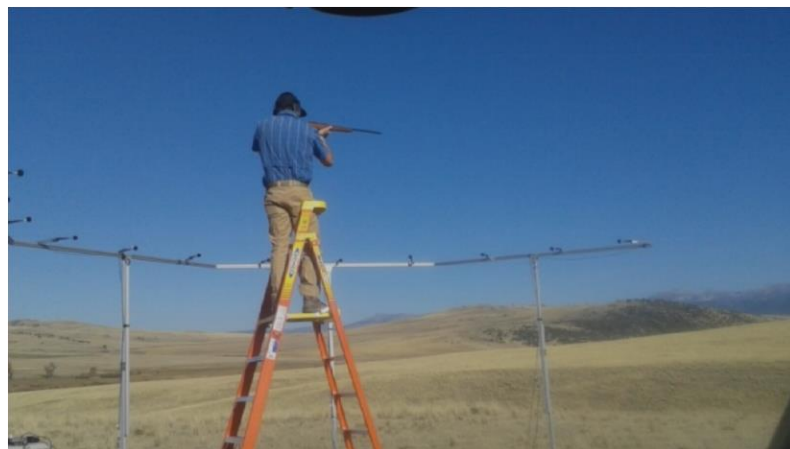
Figure 1: Shooting from an elevated platform to create time lag between the direct and ground-reflected signals
